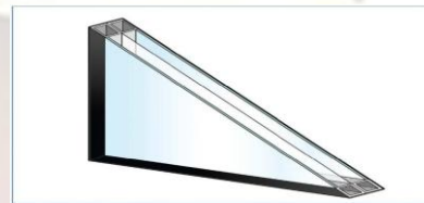
Fig 13: Cutaway of triple- pane insulated glass unit.
