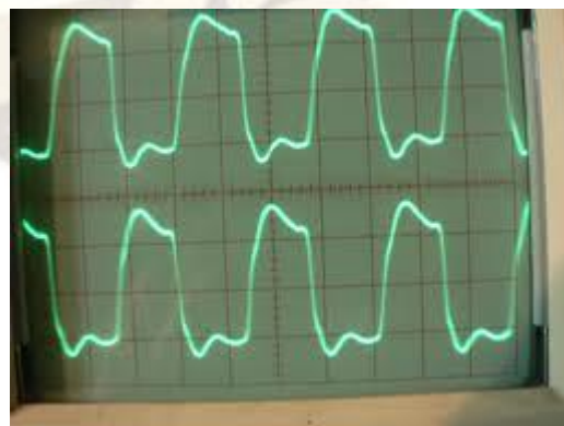
Figure4 PPG signal at 660nm LED
