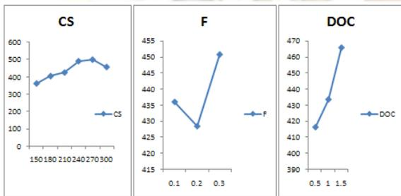
**Fig 1 Main effect plot for means of MRR**
