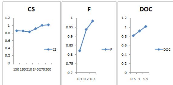
**Fig 2 Main effect plot for means of Ra**
