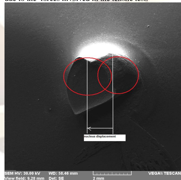
Fig. 6 Pullout failure mode of S235JR steel
