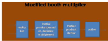
Fig 2.1 Block diagram of modified booth multiplier
