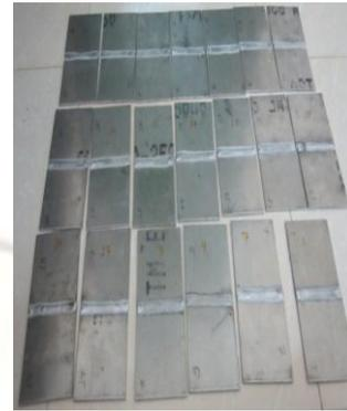
Fig. 1 Photos of Welded Specimen
