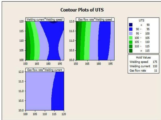
Fig.7 Contour plot for UTS
