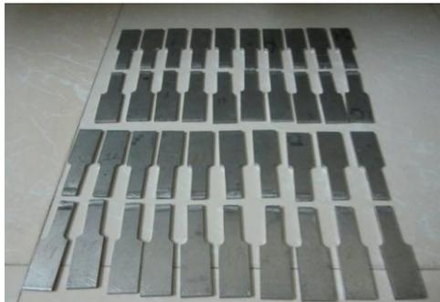
Fig.4 Specimen after tensile test
