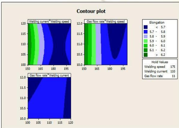
Fig 9. Contour plot for % Elongation
