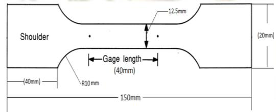
Fig.2 Dimensions of tensile test specimen
