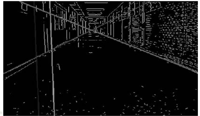
Fig. 8 Result of the Hough transform with the threshold being 0.8 the higher-order computation. In order to obtain the optimal edge detected image, the slope rate of the Gaussian function and the size of the sectioned matrix should be adjustable. Neural units with higher-order synaptic operations for robotic image processing applications 227 CCD camera image acquisition were processing & edge detection Ultrasonic, infrared, odometer & electronic compass Localization, obstacle avoidance & path routing Higher-order neural units for data fusion and image processing. Feature extraction & matching Database updating Direction & speed control.
