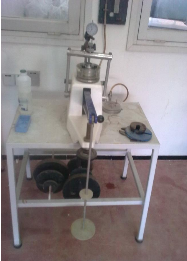
Figure 5: Equipment used in the oedometer methods.
