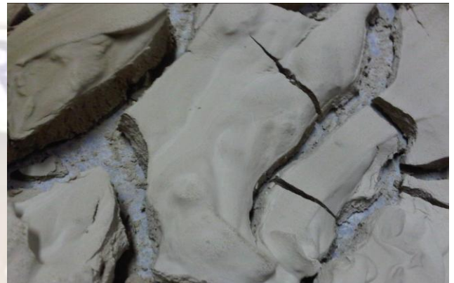
Figure 1: Green clay of Gzenaya (Tangier) after sieving to 80 \mu\text{m} in laboratory and drying.
