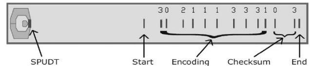
Fig. 4 Mask image of a reflector-based SAW RFID tag [10]
