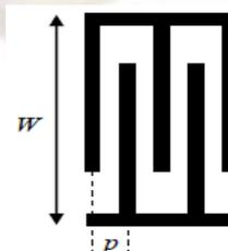
Fig.3 Interdigital transducer (IDT) [12]
