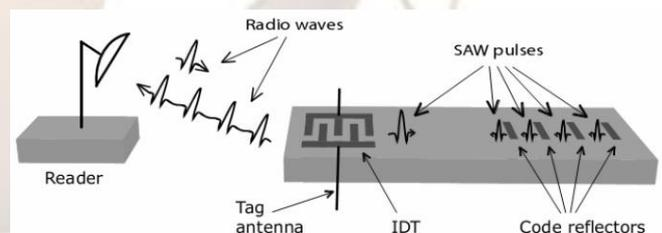
Fig.2 Operation of a SAW tag [11]
