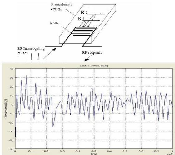
Fig.7 The design of the proposed SAW RFID tag
