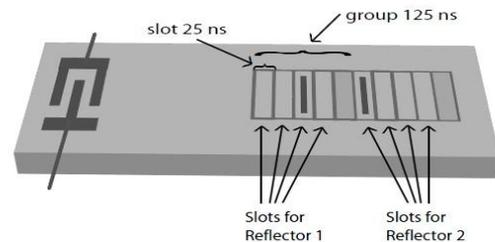
Fig. 5 Principle of time position encoding. Schematic drawing [10]
