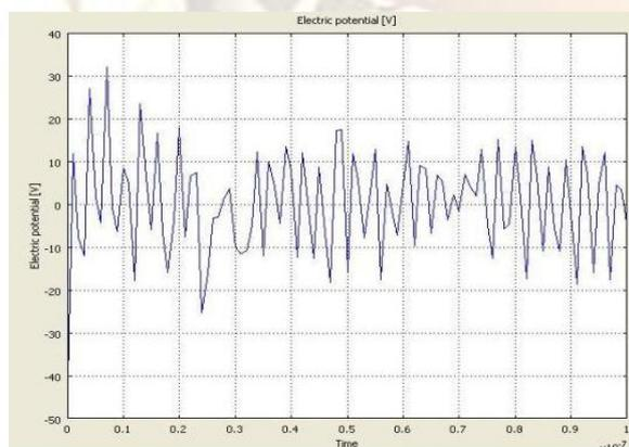
Fig.8 Therespone of the proposed SAW RFID tag
