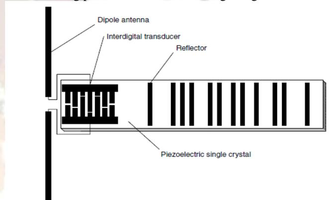
Fig. 1 Basic layout of an SAW transponder. Interdigital transducers and reflectors are positioned on the piezoelectric crystal [13]
