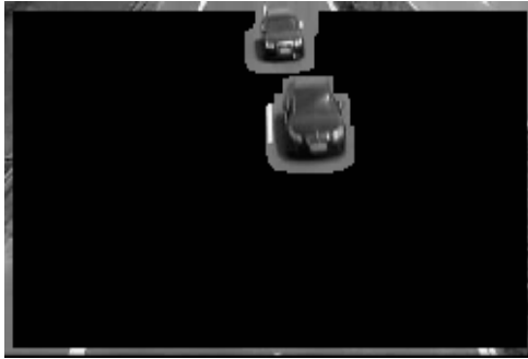
Fig.4. object detection using kalman filter method
