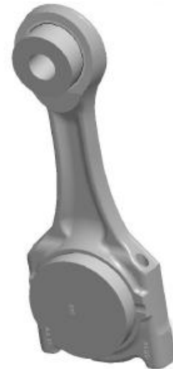
Figure 6 – Connecting rod model for FEA.
