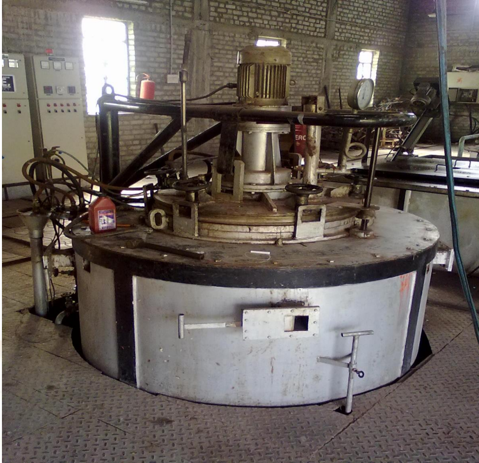
Figure 1 GAS CARBURIZING FURNACE
