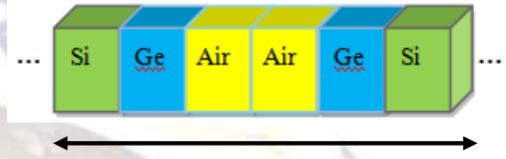
Fig. 4. Periodic structure of 501 layers with defect
