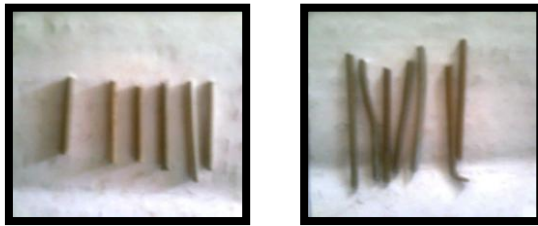
(a) (b) Figure 5.7 – 30MM Fibres (a) & 50MM Fibres (b) used for Concrete Mix [M-20]
