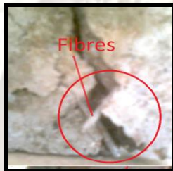
Figure 5.9 –Cube Test of Fibres Mixed Concrete
