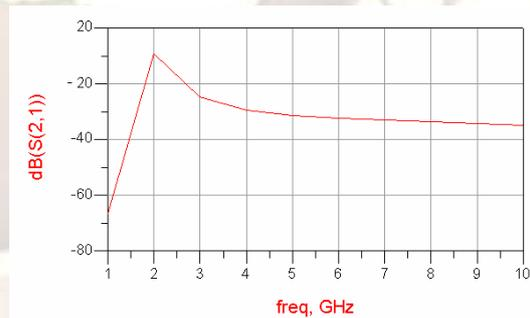
Fig 15. dB(S21) and dB(S12) Butterworth Filter With Component Element
