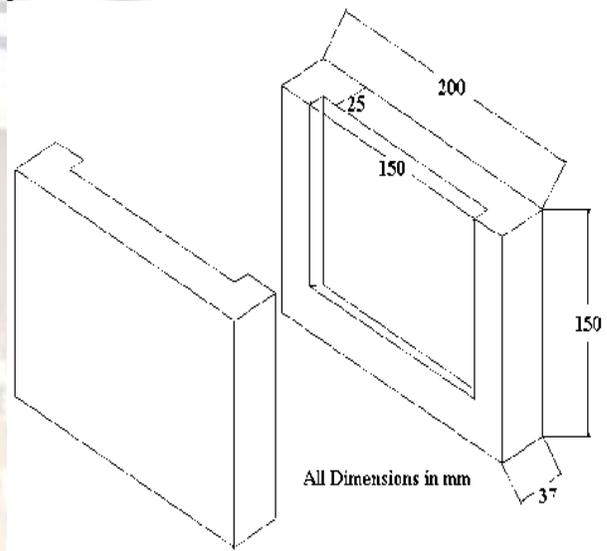
Fig.1 Cast Iron Metal Mould
