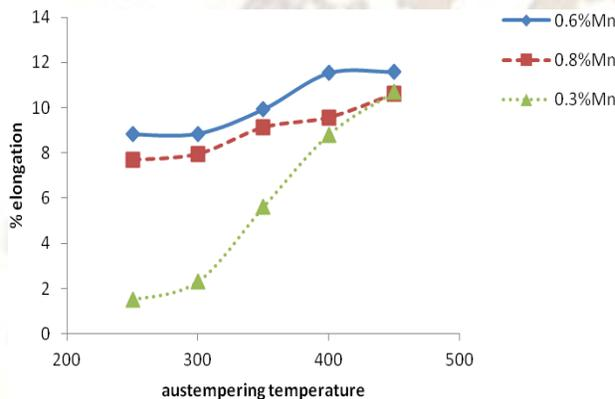
**Fig 6-1: Effect of austempering temperature on % elongation soaked for 60 min.**
