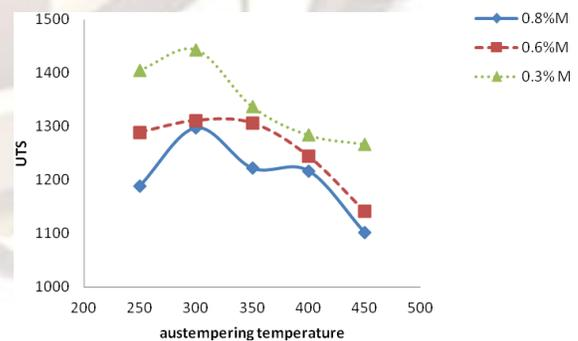
**Fig 5-3: Effect of austempering temperature on tensile strength soaked for 120 min**
