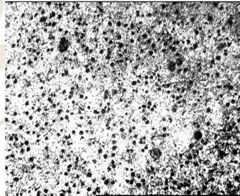
**Fig 4-4 (100X-Nital etched): Micro-Structure for 0.6 % Mn Sample Maintained at Temperature: 350°C for 120 min.**
