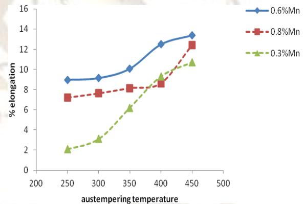
**Fig 6-3: Effect of austempering temperature on % elongation soaked for 120 min.**
