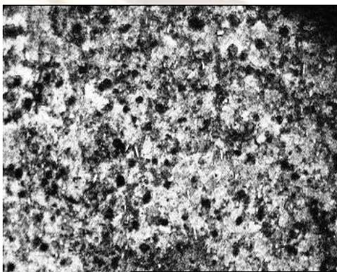
**Fig 4-5 (100X-Nital etched): Micro-Structure for 0.8 % Mn Sample Maintained at Temperature: 400°C for 120 min.**
