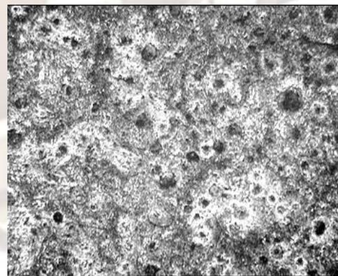
**Fig 4-6 (100X-Nital etched): Micro-Structure for 0.6 % Mn Sample Maintained at Temperature: 400°C for 120 min.**
