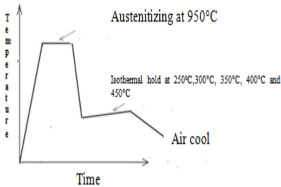
**Fig. 2: Two-step Austempering heat treatment cycle**
