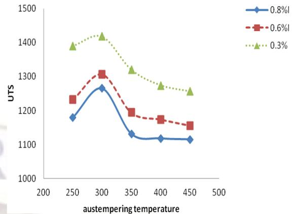
**Fig 5-1: Effect of austempering temperature on tensile strength soaked for 60 min.**
