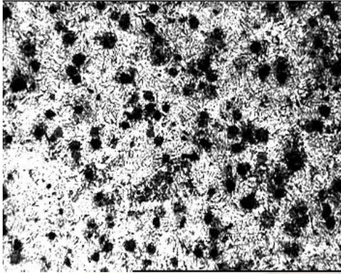
**Fig 4-1 (100X-Nital etched): Micro-Structure for 0.8 % Mn Sample Maintained at Temperature: 300°C for 120 min.**
