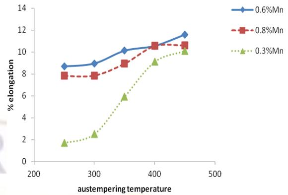
**Fig 6-2: Effect of austempering temperature on % elongation soaked for 90 min.**
