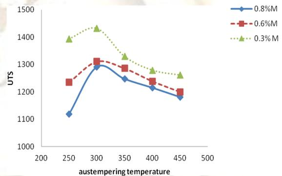
**Fig 5-2: Effect of austempering temperature on tensile strength soaked for 90 min.**
