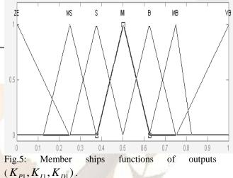
Rule base: A decision-making logic, which is, 2. simulating a human decision process, inters fuzzy control action from the knowledge of the control rules and linguistic variable definitions. The basic rule base of these controllers' types is given by:
