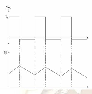
Fig.7: Pulse width modulation.
