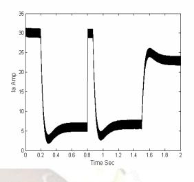
Fig.9.a: Motor current  $I_a$  using conventional PID
