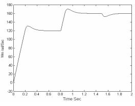
Fig.9.c: Motor speed  $\omega_m$  using conventional PID controller.
