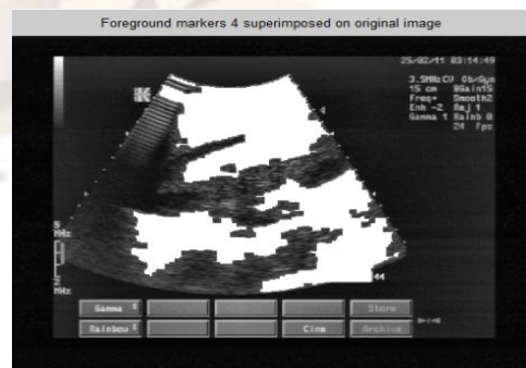
Fig. 7: Advance foreground marked after applying “ bwareaopen ” function.
