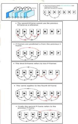
Figure 2: The above figures show how I,B,P Frame work
