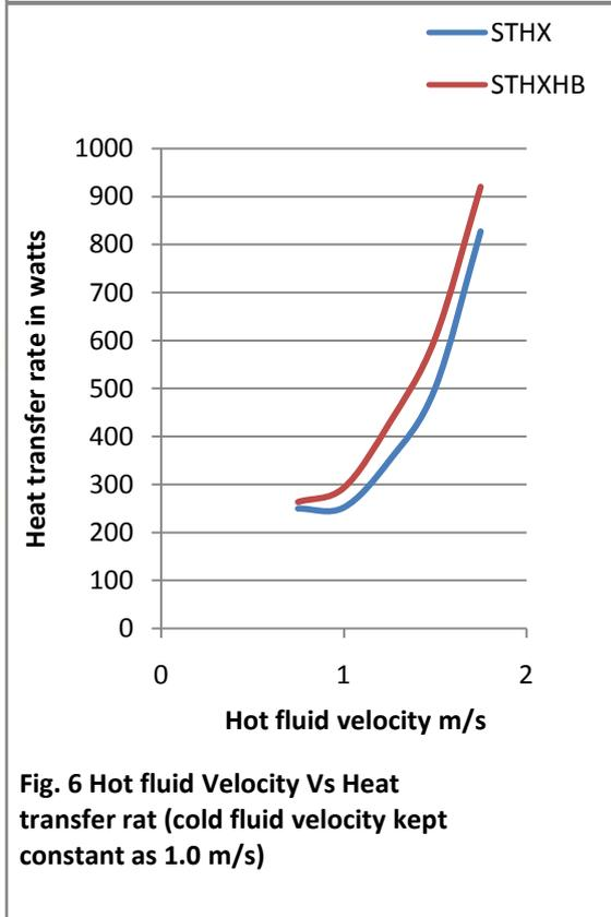
Fig. 6 Hot fluid Velocity Vs Heat transfer rat (cold fluid velocity kept constant as 1.0 m/s)
