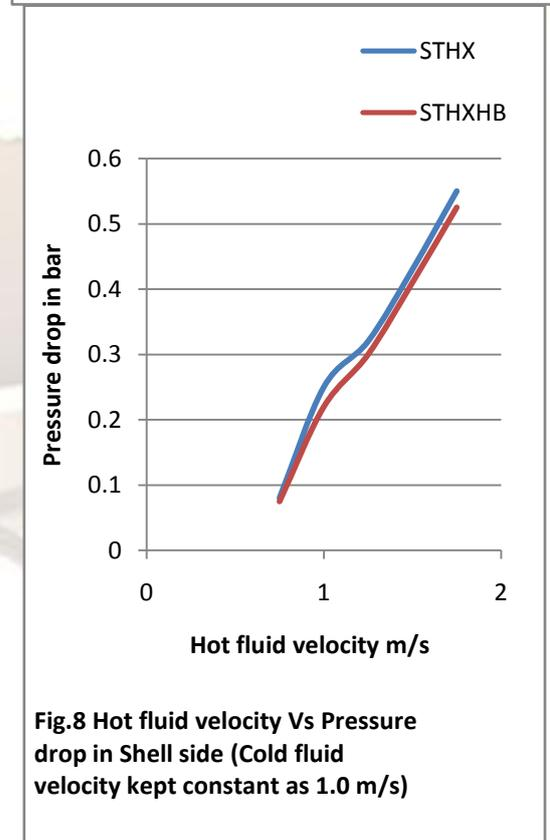
Fig.8 Hot fluid velocity Vs Pressure drop in Shell side (Cold fluid velocity kept constant as 1.0 m/s)
