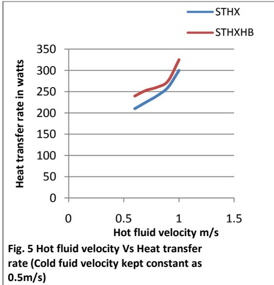
Fig. 5 Hot fluid velocity Vs Heat transfer rate (Cold fluid velocity kept constant as 0.5m/s)
