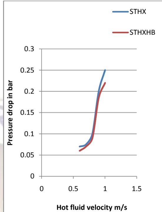
Fig. 7 Hot fluid velocity Vs Pressuredrop in shell side (Cold fluid velocity kept constant as 0.5 m/s)
