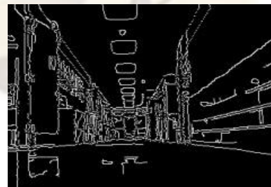
Figure 4. Edge detection on an un-blurred image
