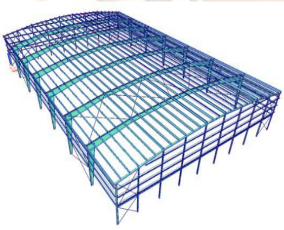
Fig: 4. Pre-Engineered Building
