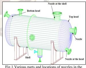
Fig.1.Various parts and locations of nozzles in the vessel
