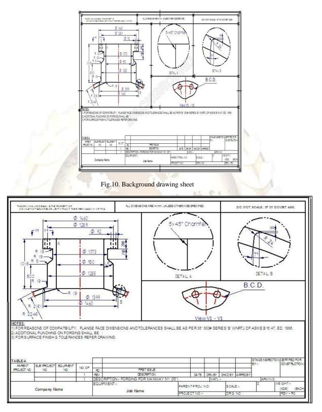
Fig.11. Manufacturing nozzle drawing sheet
