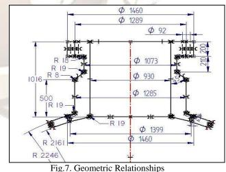
Nozzle main parts Nozzle ID, Hub Height, Hub OD, Neck OD, Bolt Hole Dia., Flange OD, BCD, Flange Height, Neck height, Lip Height, Lip Radius, Lip Angle, Chamfer, Chamfer Angle, Lip OD, Lip
