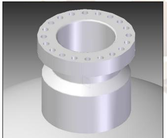
Fig.4. Nozzle on Head (Isometric view)
