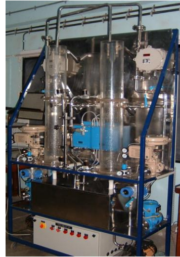
Figure 3 Actual Four tank Setup
