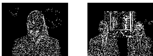
Fig 2. (a) Frame difference between 54 th and 56 th (b) Frame difference between 2 nd and 4 th
