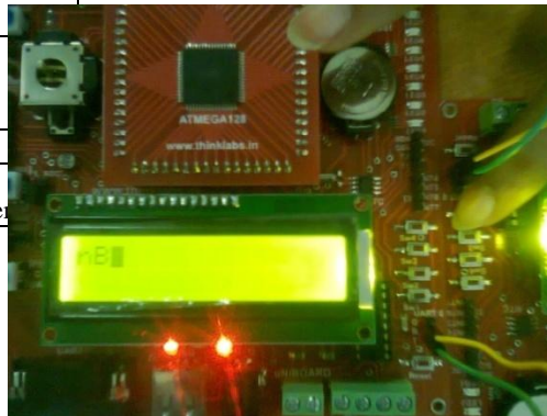
Fig.3-O/P when switch 1 is pressed
