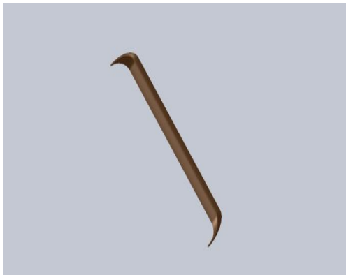
Fig. 3.1 Shows geometric model of section of Shell with Head. Having uniform thickness 6 mm.
