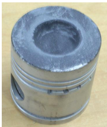
Figure 2 Piston with Sic coating using Plasma Spray Process
