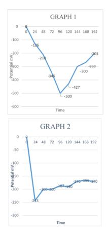
The above results, the corrosion is occurs highly in non-protective concrete. The protective concrete, the rate of corrosion is low. The stable oxide layer is forming on rebars. The stable layer was reduced the corrosion rate in rebars. In anodic protected concrete, the corrosion is controlled by zinc.
