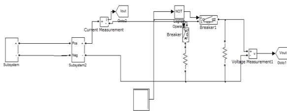
Fig.12 MATLAB/Simulink model of full bridge converter with step change in load
