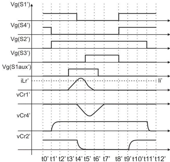
Fig.10 operating waveforms
