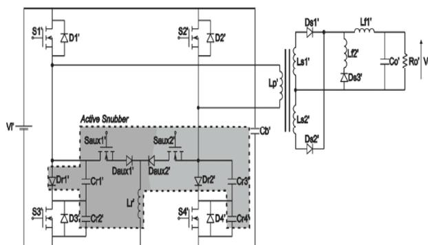
Fig. 1 Full bridge soft switched dc-dc converter with non-dissipative snubber.
