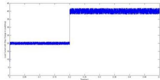
Fig.16 Load Current with step change of load at 0.25 sec.
