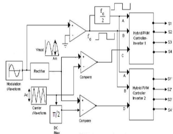
Fig 12: Hybrid Phase-Shifted Carrier PWM Technique (HPSC)
