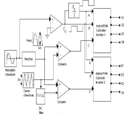
Fig 9: Hybrid Alternative phase opposition Disposition (HAPOD)
