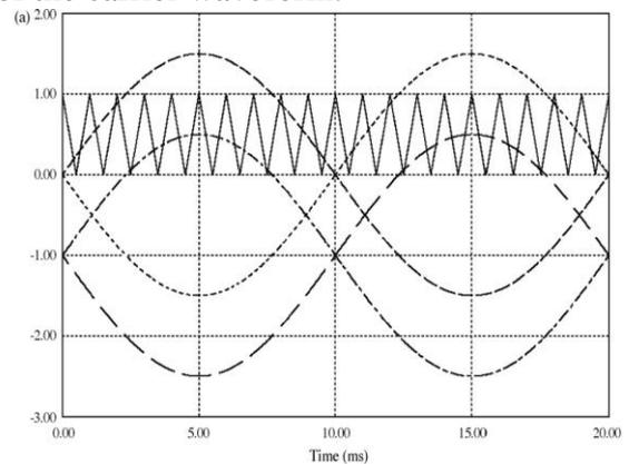
Fig 5: One carrier and two reference signals
