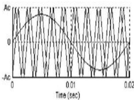
Fig 4: result for (five-level) PSC operation
