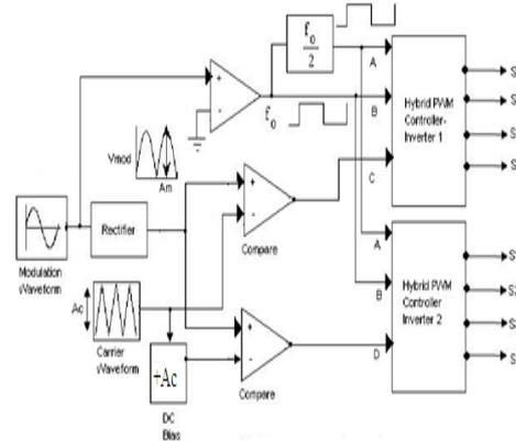
Fig 11: Hybrid Carrier-Based Space-Vector Modulation (HCBSVM)
