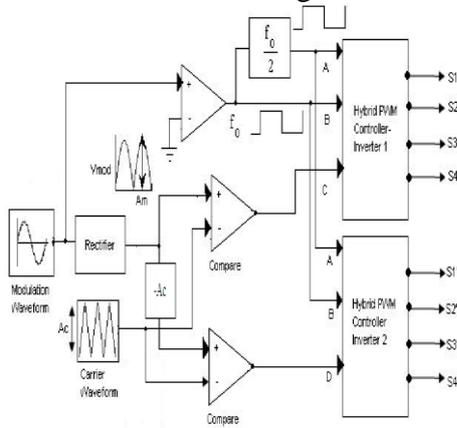
Fig 10: Hybrid Single-carrier sinusoidal PWM (HSC-SPWM) technique
