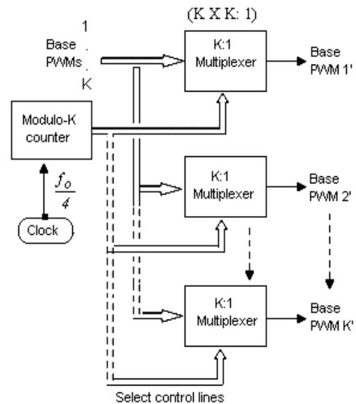
Fig 14: Scheme of base PWM circulation for  $N$ -level operation
