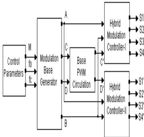
Fig 8: proposed sequential hybrid modulation
