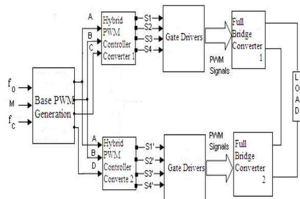
Fig 7: Hybrid Modulation SchemnBase Modulation Design
