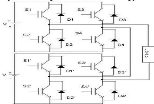
**Fig 1: Schematic diagram of the inverter topology**
