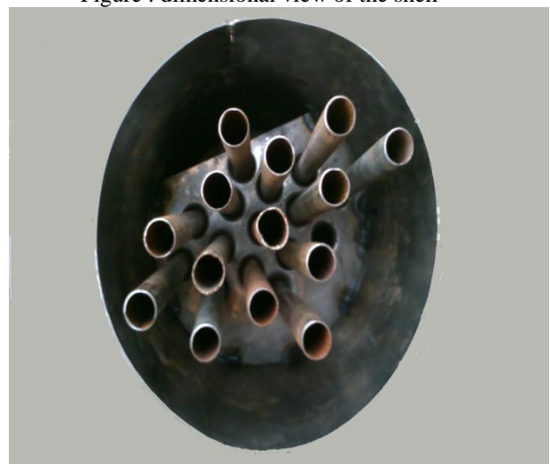
Figure :Shell with Tubes and baffle during manufacturing Internal View:
