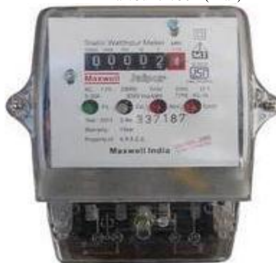
Figure 6. AC 1ph, 2 wire static wathour meter.
