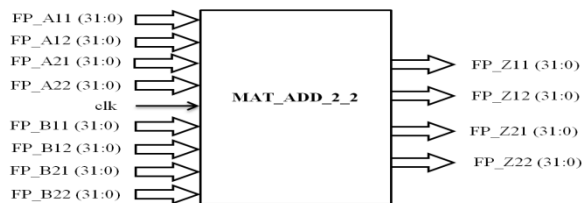
Figure 5: Block Diagram of 2x2 Matrix Addition
