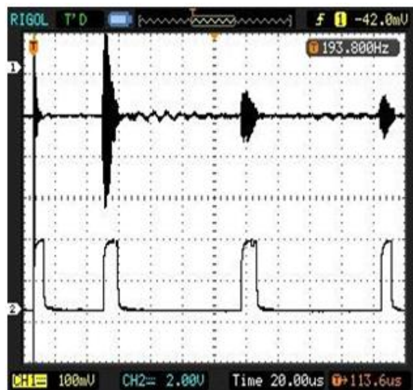
Fig. 10 Snapshot of received echoes with single pulse conversion
