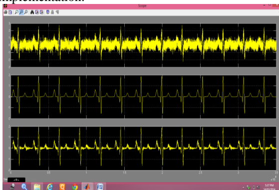
Fig.2. Simulation of ECG signal corrupted with impulsive noise and its suppression using LMS algorithm
