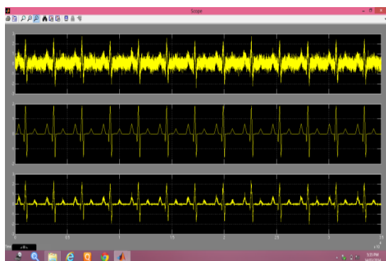
Fig.3. Simulation of ECG signal corrupted with noise and its suppression using new approach.
