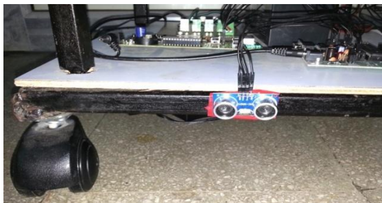
Fig 8: Ultrasonic Sensor mounted at the base
