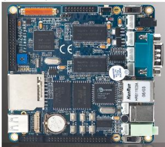
Fig2. Mini2440 Development board
