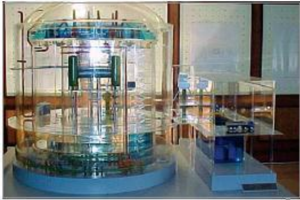
Fig 4: Scaled Model (1:50) of AHWR Acrylic Material
