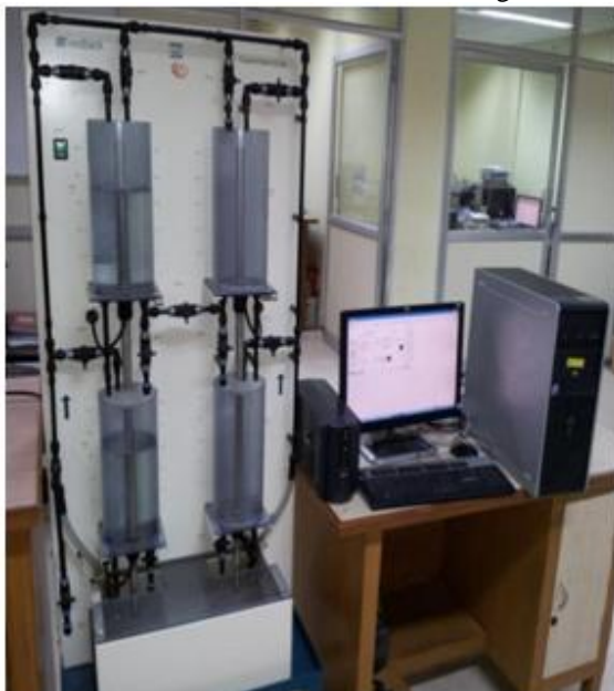
Fig.2. Experimental set up of Coupled the Tank System
