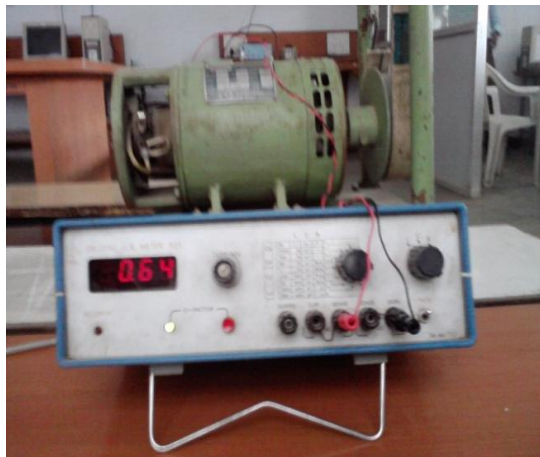
Figure.5.: Experimental arrangement for measurement of Ra and Lf of SEDC Motor
