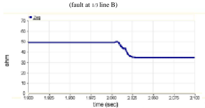
Fig. 14. Measured apparent impedance in point A in presence of TCSC (fault at 1/3 line B)
