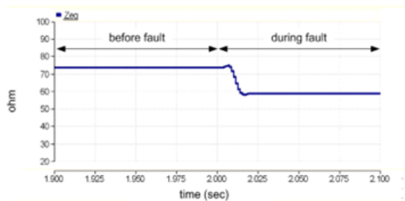
Fig. 10. Measured apparent impedance in point A without TCSC (fault at 2/3 line B)
