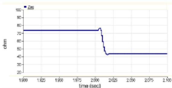
Fig. 11. Measured apparent impedance in point A without TCSC (fault at 1/3 line B)
