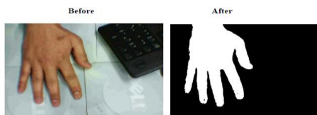
Fig. 5 Removal of Background
