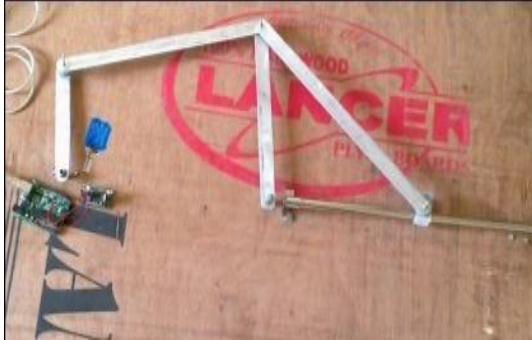
Fig.5. Actual Model of Compound linkage Mechanism
