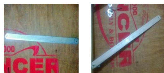
Fig.4. Rocker and connecting rod
