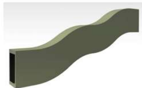
Fig.1 Double –S duct set up
