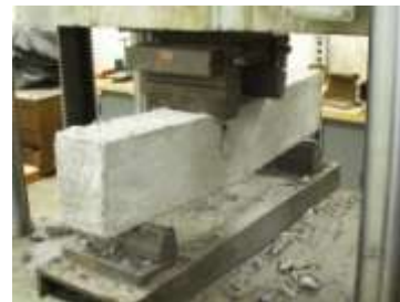
Flexural Testing of Specimen
