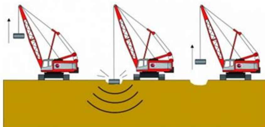
Figure 7 Dynamic Compaction process
