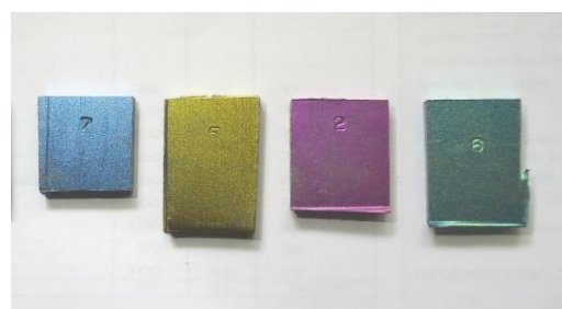
Fig. 2.4: Titanium Spectrum at different voltage ranges in KOH bath [22]
