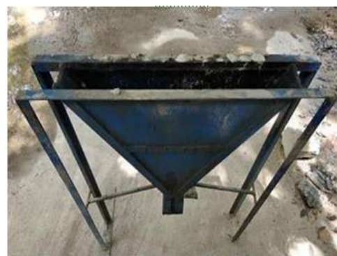
Fig 3 prepared V-funnel as per EFNARC guide lines
