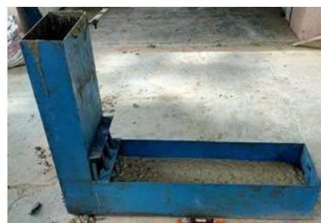
Fig 4 Shows the flowing concrete through reinforced bars in L-box after lifting gate
