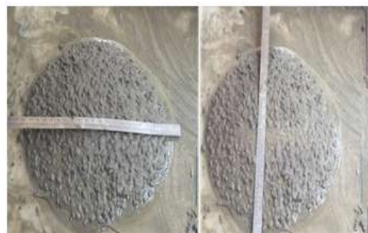
Fig 2 Measuring the slump flow of D1 and D2
