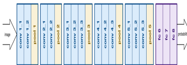
Figure 2: The VGG16 architecture
